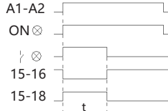
type A delay time sequence chart
